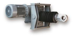
Maximum loads of up to 350 kN can be realised with the linear actuator employed, a BJ4, while a maximum static load of 500 kN (BJ5) is possible with the BJ series. The complete universal joint is made of galvanized steel with a triple coat of lacquer. A basic version was supplied. The spindle is protected by a bellows so that no dust or dirt can penetrate into the actuator.
