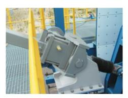
not rigid, but must be capable of being swivelled – in both the X and Y direction. This allows the baffle flaps to be adapted to the type and quantity of material being conveyed.
